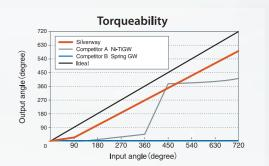
inserted into a looped catheter and the proximal shaft is rotated. The length from the tip to the machine is kept equal.
